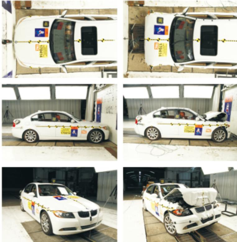
Figure 2 FMVSS 212 Test Data
